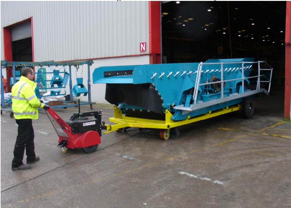
Powerscreen International Manufacturing Engineer, Stuart Adair, using the Nu-Star Super Pusher to manoeuvre the 6,500Kg screen box sub-assembly
