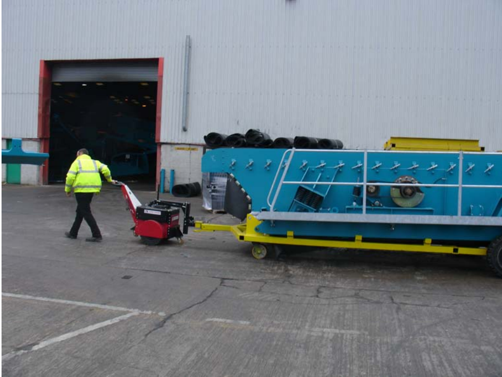
Powerscreen International Manufacturing Engineer, Stuart Adair, using the Nu-Star Super Pusher to manoeuvre the 6,500Kg screen box sub-assembly
