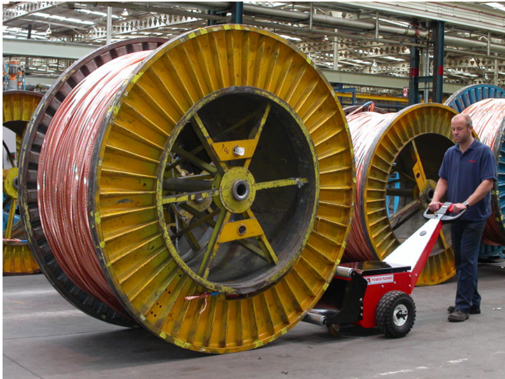
Stuart Chetwyne (Pirelli Cables, Wrexham) pushing a 9 tonne cable drum with the Nu-Star Power Pusher
