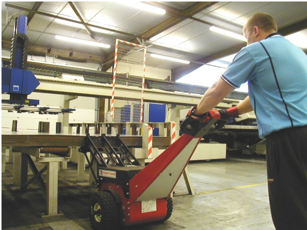
Permastore's Kevin Woods with the Power Pusher to feed steel sheet in to the Trumpf press
