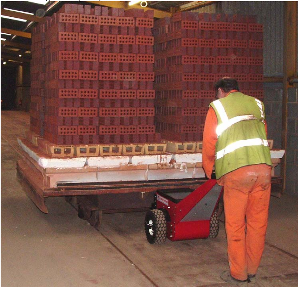
Neville Smith using the Power Pusher to push one of the 12 tonne brick kiln cars at Hanson, Halifax
