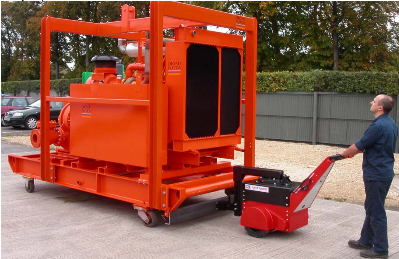
Richard Godwin using the Nu-Star Super Pusher to manoeuvre one of the 4800Kg Godwin Pumps
