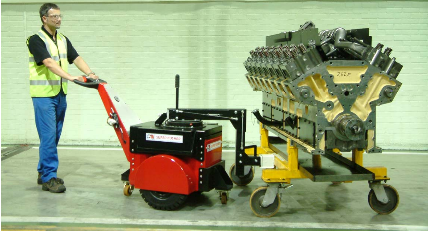
Eddie East using the Nu-Star Super Pusher to manoeuvre one of the 7000kg KV16 diesel engines
