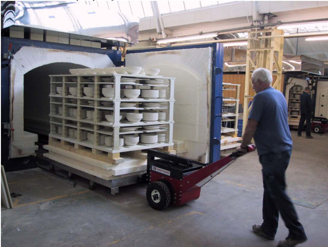
Harry Hunt (Churchill China plc, Stoke-on-Trent) pushing a 2 tonne kiln car into the oven with one of the Nu-Star Power Pushers
